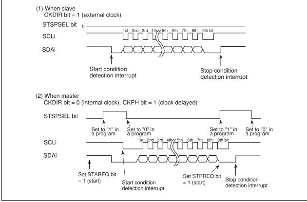
Figure 14.26 STSPSEL Bit Functions
